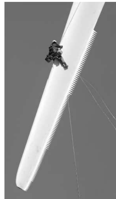
GE prototype turbine with trailing edge serrations
